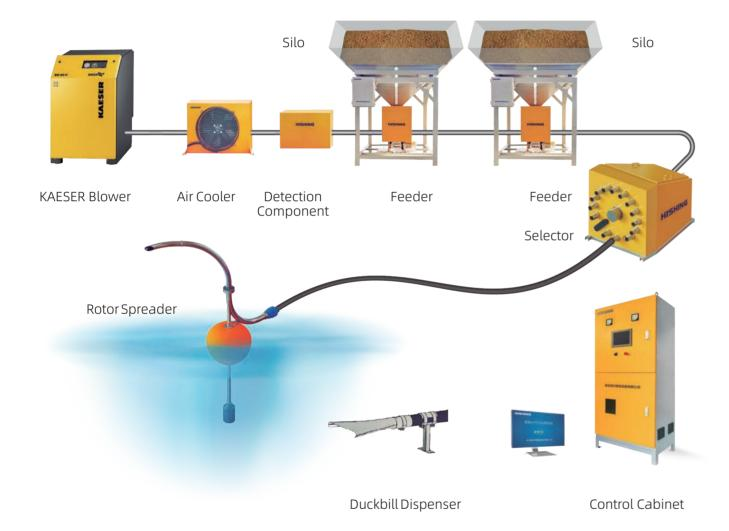
Smart pneumatic feeding system is an advanced centralized feeding system, suitable for multiple types of aquaculture, such as sea cages, fresh water cages, RAS, and pond aquaculture, etc.
