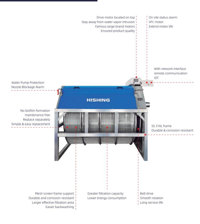
Mesh screen as the medium, SMART drum type filter removes the tiny solid in water by mechanical physical filtration directly. It can quickly, massively and effectively filter the pellets, feces and organic particles, cooperating with other equipment, it can complete series treatment such as filtration, disinfection, sterilization and oxygen enrichment for the recirculating water.
